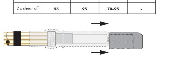
After tightening the contact, slide the cable reducer up until it butts against the contact.
