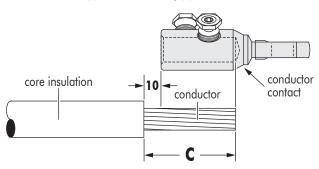
For mechanical type contacts: remove the core insulation from the conductor for a distance « C » mm (C = depth of contact bore + 10 mm).
