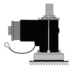
Tighten the butterfly nuts, be careful not to apply excessive force. The KAA4/8 adapter must be perfectly positioned on the interface of the bushing.
