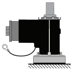
Place the metal mounting plate on the shoulder of the male part of the KAA4 adapter.
